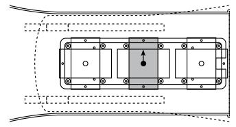
Figure 25 – Proper Stinger Mount position for measuring wing lift
