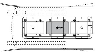
Figure 26 – Proper Stinger Mount position for measuring wing or geometric shape drag
