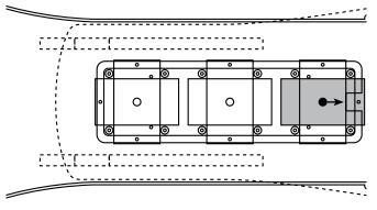
Figure 27 – Proper Stinger Mount position for measuring rocket drag
