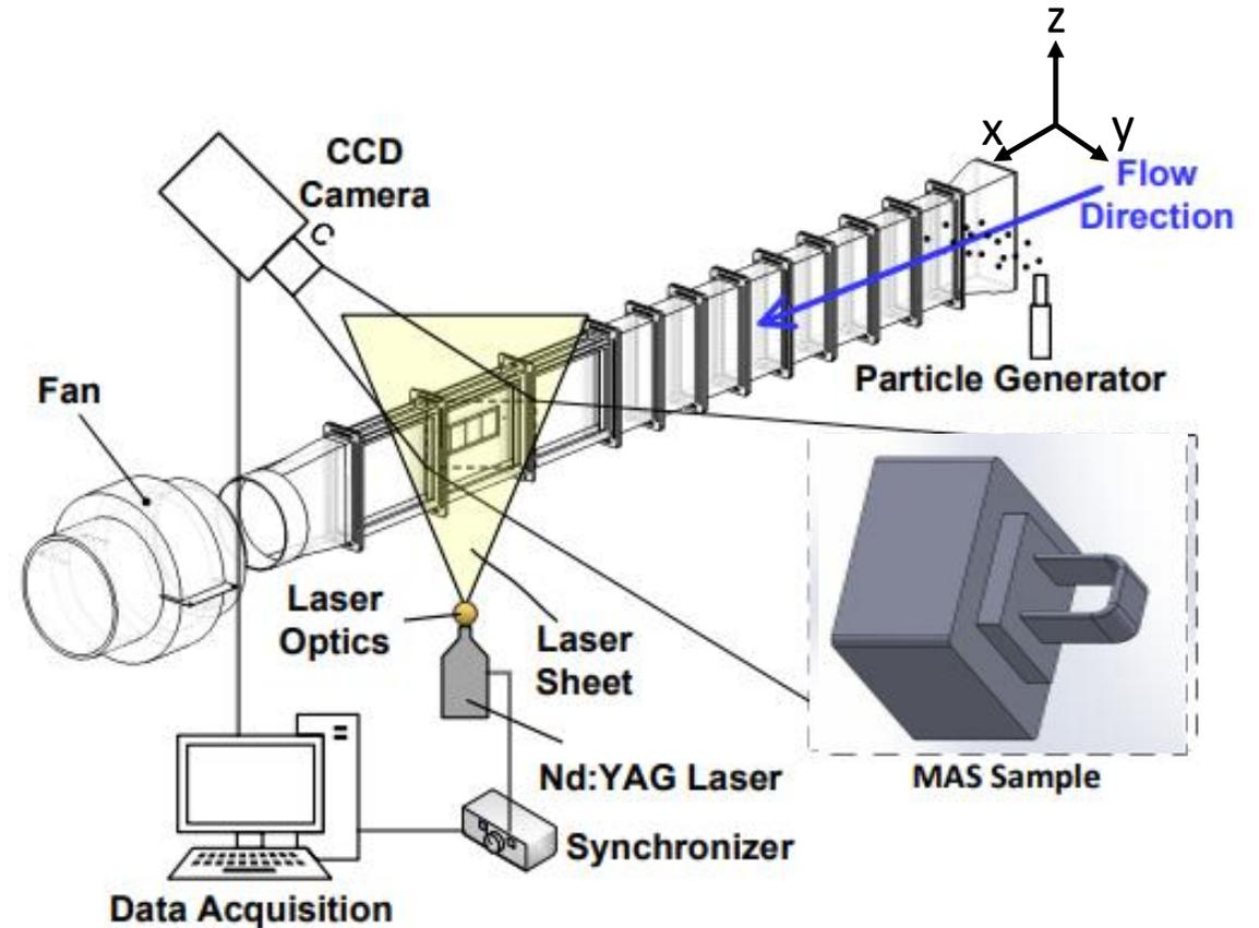
Schematic of Wind Channel/PIV Setup
