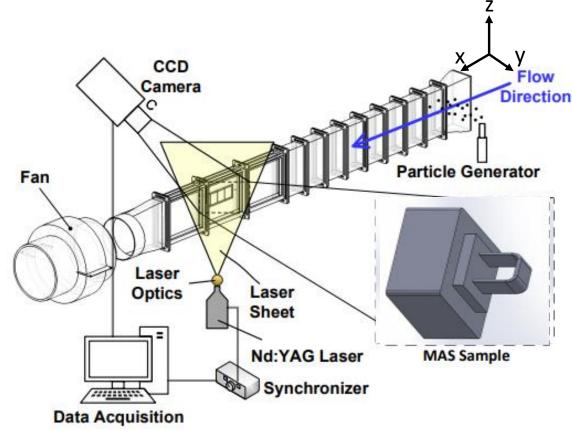
Schematic of Wind Channel/PIV Setup
